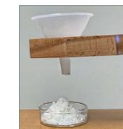
Fig 5: Angle of repose experiment
